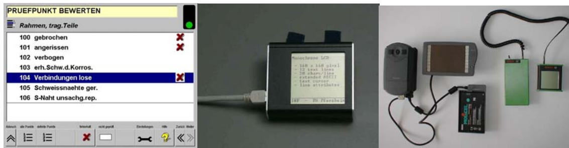
Figure 4 (left to right) SCWC 1 graphical user interface, text-based LCD display of SCWC 2, hardware comparison of SCWC 1 (left in third image) and SCWC 2
