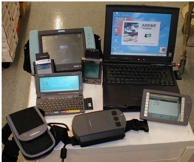
Figure 1: Clockwise from top right: Acer laptop; touchscreen, CPU unit, and battery of Xybernaut MA IV wearable computer; Sharp handheld; Compaq iPaq and Casio Cassiopeia PocketPCs; and Siemens Mobic Pentablet PC.
